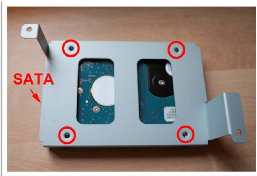
4. Insert the hard drive rack with the installed hard drive with the two screws. Connect the power cable from the power supply and the red SATA-cable as shown below.
